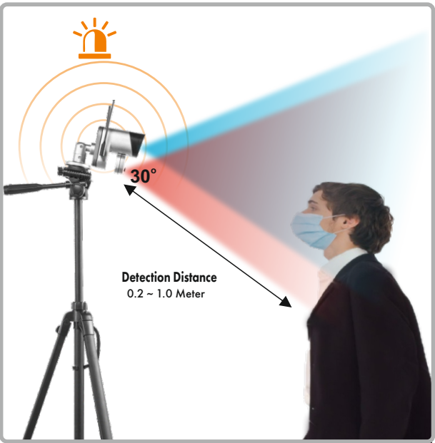
Camera detects human body and voice prompts the person to stand within detection area for measuring body temperature.
